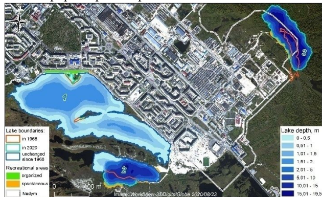
Figure 5. A bathymetric survey (depth) of the largest natural and artificial bodies of water (lakes and dugouts) and lake recreational areas. The organized recreational area has been developed by the municipality; the spontaneous recreational area lacks municipal funding and has been developed by urban residents themselves.
